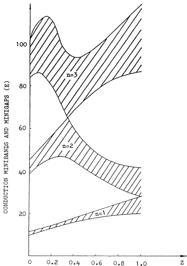
FIG. 2. The first three allowed conduction minibands (shaded area) and minigaps as functions of  $Z$  ( $= b_2/b_1$ ) for  $L = 150$  Å,  $a_1 = a_2 = 15$  Å, and  $x = 0.3$ . The energy unit  $E$  is  $\hbar\pi^2/2m_eL^2$  (1.67 meV).
