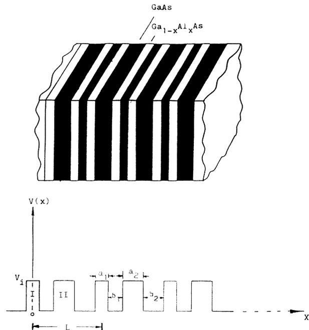
FIG. 1. Schematic superlattice. (a) Compositional superlattice consisting of double layers of GaAs and Al<sub>x</sub>Ga<sub>1-x</sub>As materials per period. (b) Band profile of the superlattice showing the periodic potential arising from the band-gap difference between GaAs and Al<sub>x</sub>Ga<sub>1-x</sub>As.
